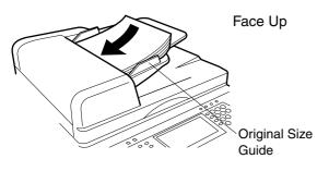
• Insert the original(s) Face Up into the ADF until the leading edge placed into the machine stops.
